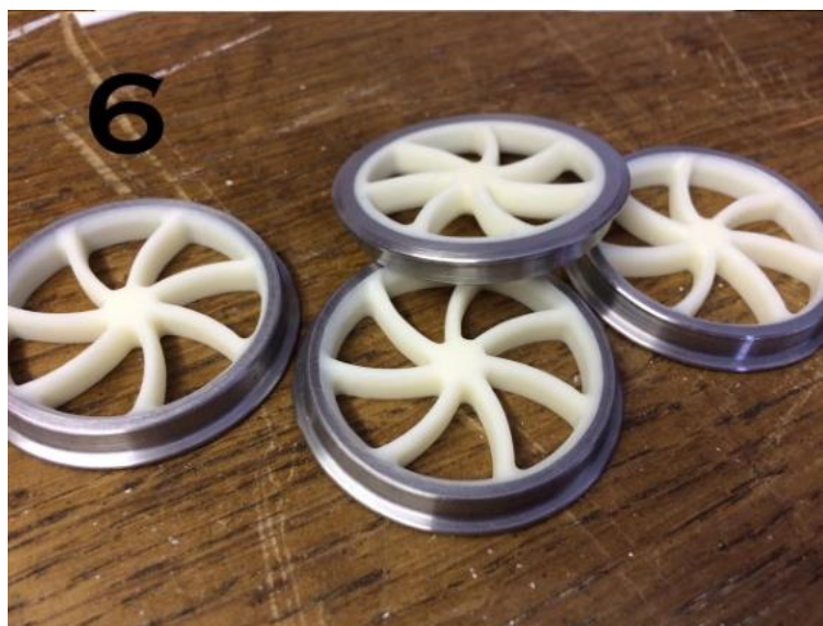
Photo 6 : When the resin is set, pop it out of the mould and repeat. The excess resin on the backs of the wheels is sanded off until flush with the tyre.
