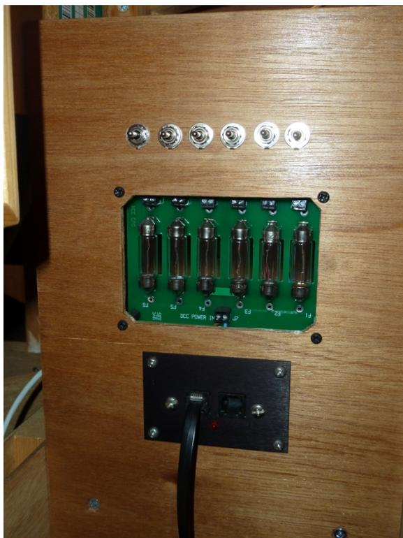
The five section switches are at the top. (Yes, I know there are six, but that is for any future change of plan). In each case the centre position, as shown, is *off*, and down is *on*; except for the left hand section 1 switch where centre is *off*, down is *on* for DCC, and up is *on* for DC. The cable at the front connects to the Powercab, and the H&M controller is wired in at the back. That is all there is to it. Oh really - so what is that green board in the middle with the tubes on it?
