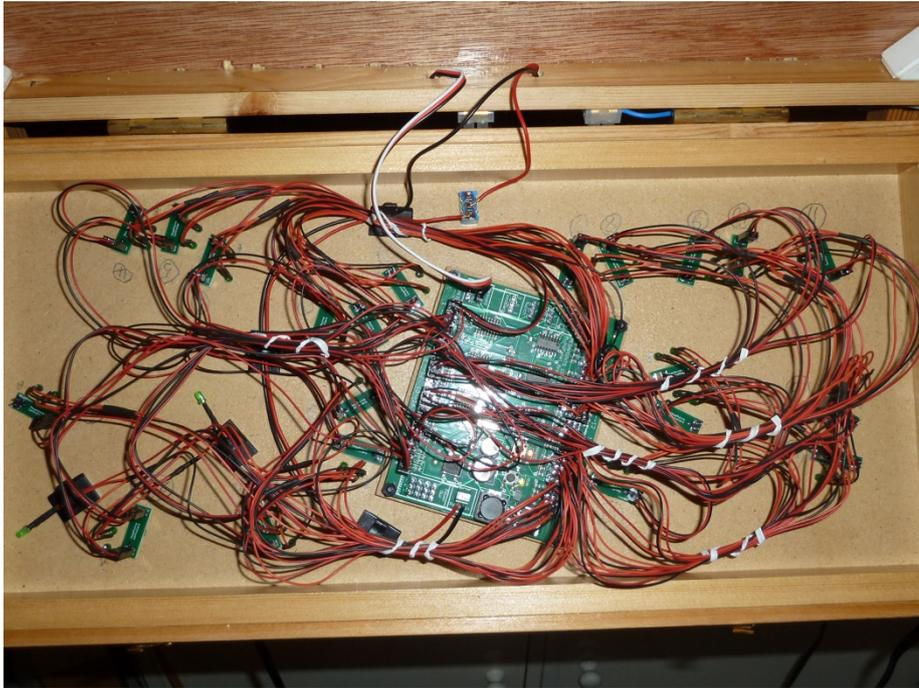
It is not nearly as complicated as it looks – honestly! The pre-wired switches and LCDs plug into the Megapoints master board. One lead brings in power, and one lead goes from here to the two point servo control boards. Each control board controls 12 point servos, and, as I have 23 servos to drive, I have two control boards. (Luckily, it was not 25!) From the control boards a three-strand cable goes to each point. Finally, here is a picture of a control board, inside and out:-
