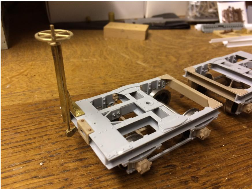
My bogies started out as a Slaters kit of mostly styrene, which I am modifying with brass bits and plasticard. The front bogie will have the brake stand, but I have upgraded the structure to be a brass one rather than the plastic one in the kit so it is stronger. The back bogie I have re-worked the brake components and made a new horizontal bracket based on photos in a WDLR book.
