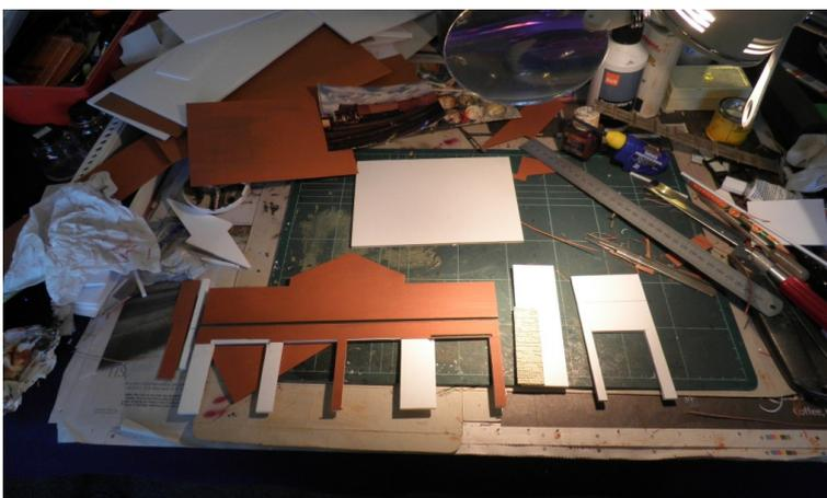
Basically, the same process was followed for the sides and ends. I was fortunate that the south side of the shed had a stepped profile in plan view, a legacy of the steam shed that pre-existed the 1950s one I was building. These steps added significantly to the structural rigidity of the model and the basic shell of the walls and ends was complete. (It is always good practice to work on a clear and tidy work table...)
