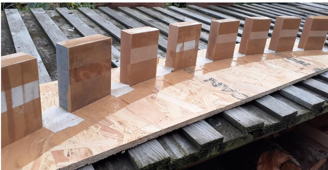
The former was made by gluing and screwing thick blocks of mdf onto a piece of OSB (Stirling board) following a 4 foot 6 inch radius curve. I was using the inside curve of the blocks, so I stuck parcel tape to prevent the glued joint between the sheets of hardboard getting stuck to the former. (If you want a straight wall, you could just use thicker plywood instead of laminating.
