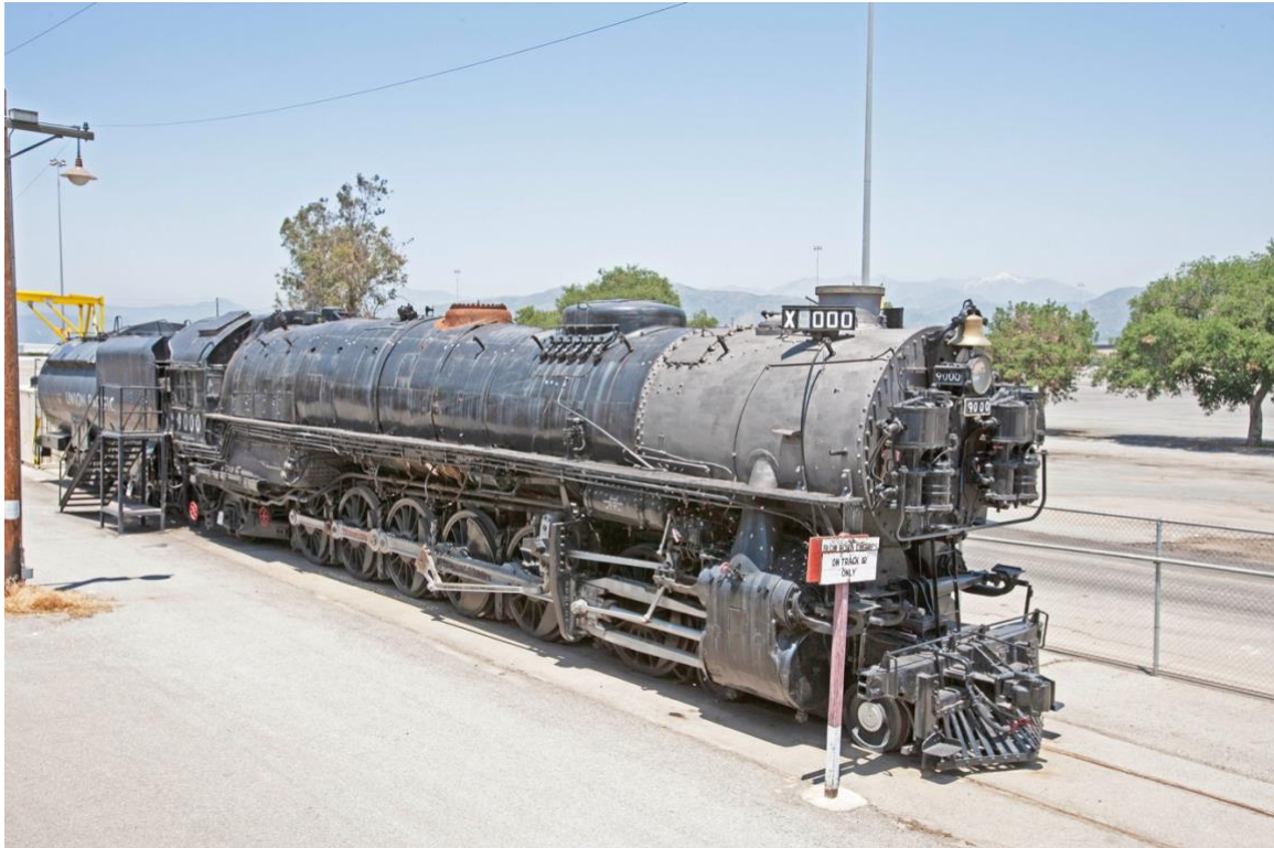
The UP 3 cylinder 4-12-2s evolved in the 1920s to haul fast freights across the vast plains.
