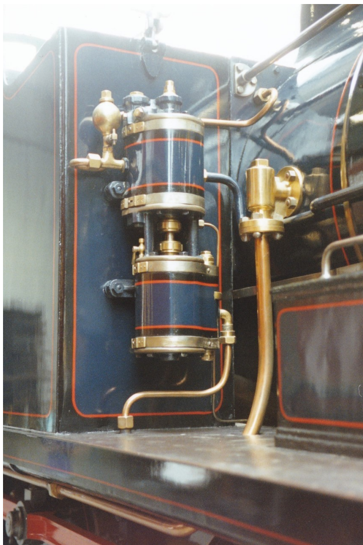
The Westinghouse pump on GER 0-6-0 tank no. 87 from the NRM collection.
