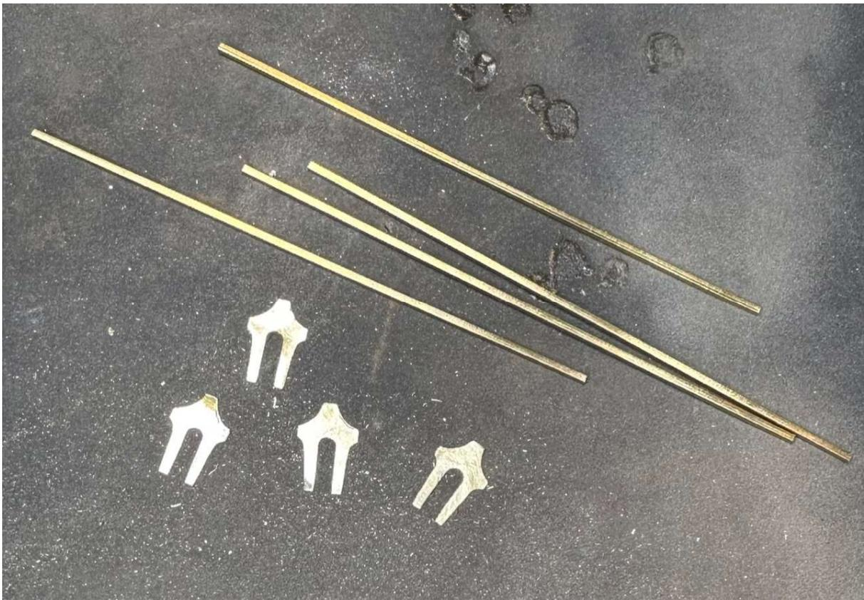
Fig.08. Four lengths of 1mm square brass rod were cut together with four axleguards cut and shaped from 10thou brass sheet. These were soldered together to form a pair of underframe sides.
