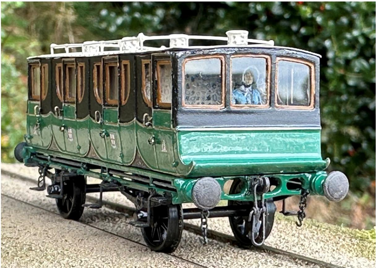
Fig.12. The windows were glazed with clear styrene with the exception of the coupé ends which use microscope glass cover slips. I used these on the recommendation of fellow Shrewsbury Railway Modeller, Stephen Duffell, and I must say the finish is far better.
