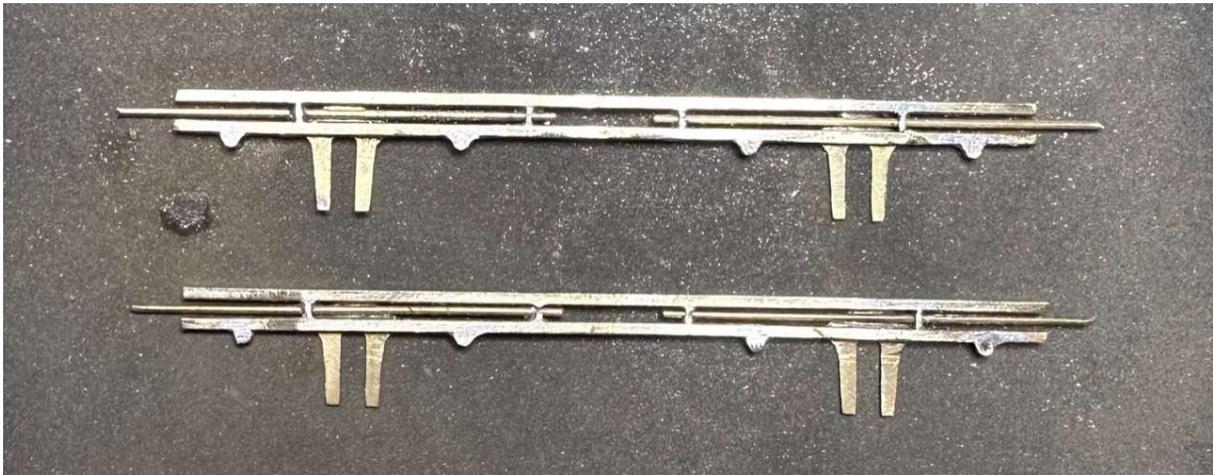
Fig.09. Guide plates for the buffer shafts were formed from 0.45mm wire bent and soldered in place before filing back flush, and 0.45mm nickel silver buffer rods were added. Roller boxes for the ends of the springs were cut from brass tube and soldered to the underside of the bottom frame.
