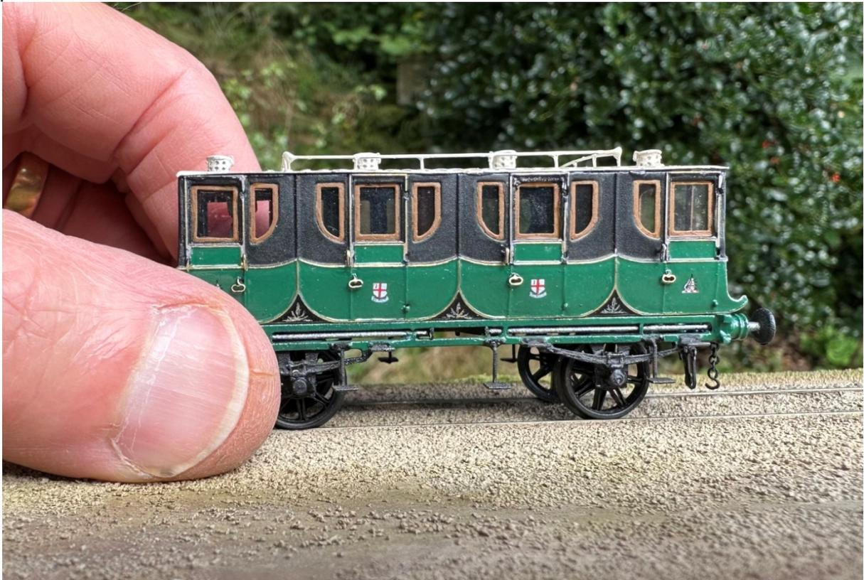
Fig.11. I chose to paint the body and apply transfers before uniting it with the underframe as it remains easier to handle as a separate unit.
