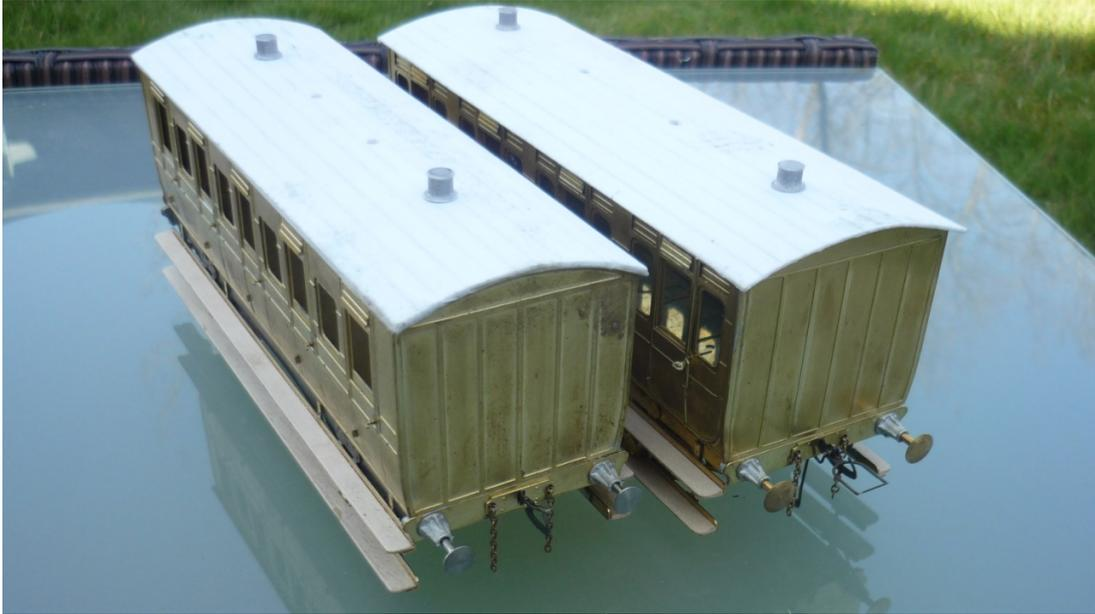
The narrow gauge wagons are fitted with a modified Spratt and Winkle which also has a pivoting latch over the top of the hook. The coupling hook engages with the bar under the adjacent wagon in the normal manner, but when drawn down by the magnet the latch will drop in to place over the hook and prevent the coupling from re-engaging when the magnet is released.
