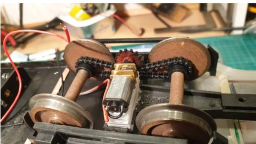
Motorising the railcar was a bit more challenging! Motor bogies in this scale can be rather expensive so I needed to come up with another method. In another project I used a small motor / gearbox unit from ebay (£2ish) which, with some gears and Delrin chain
